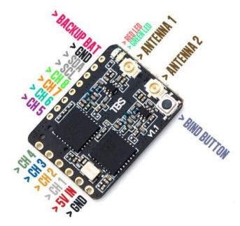
Output CH1 to CH8 are multi purpose and support the below functionality.
