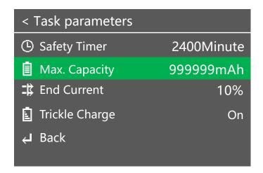
In the standby interface, Long press the speed shuttle key to pop up the "Charger Settings" menu. and then choose "Task parameters" item, the menu items are as follows:
