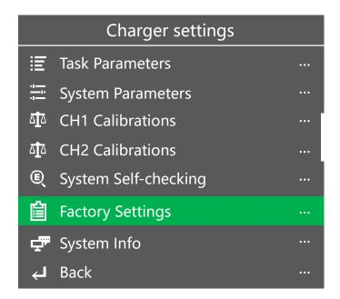
In the standby interface, Long press the speed shuttle key to pop up the "Charger Settings" menu. The menu items are as follows:
